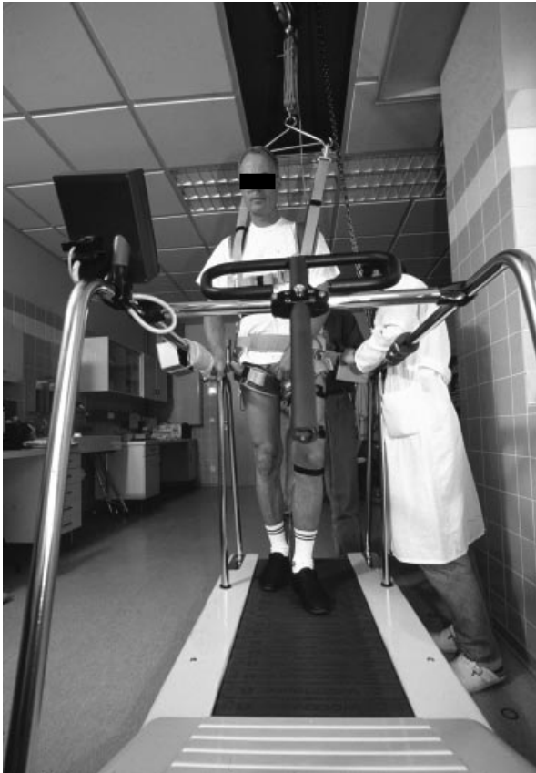
Figure 2 The treadmill trainer with partial body weight support. The treadmill is driven by a motor with variable speed control (0.01–2.25 m/s). The patient stands on the treadmill and is supported in a modified parachute harness, suspended by pulleys.
