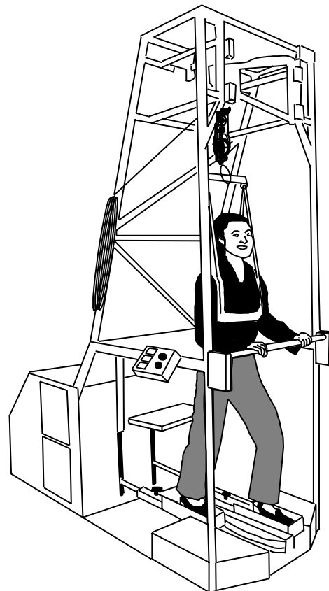
Figure 8 In the gait trainer, the patient is supported in a harness and their feet are placed on motor-driven foot plates. The machine takes the patient through a physiological gait cycle, enabling them to practice their gait many times over.
